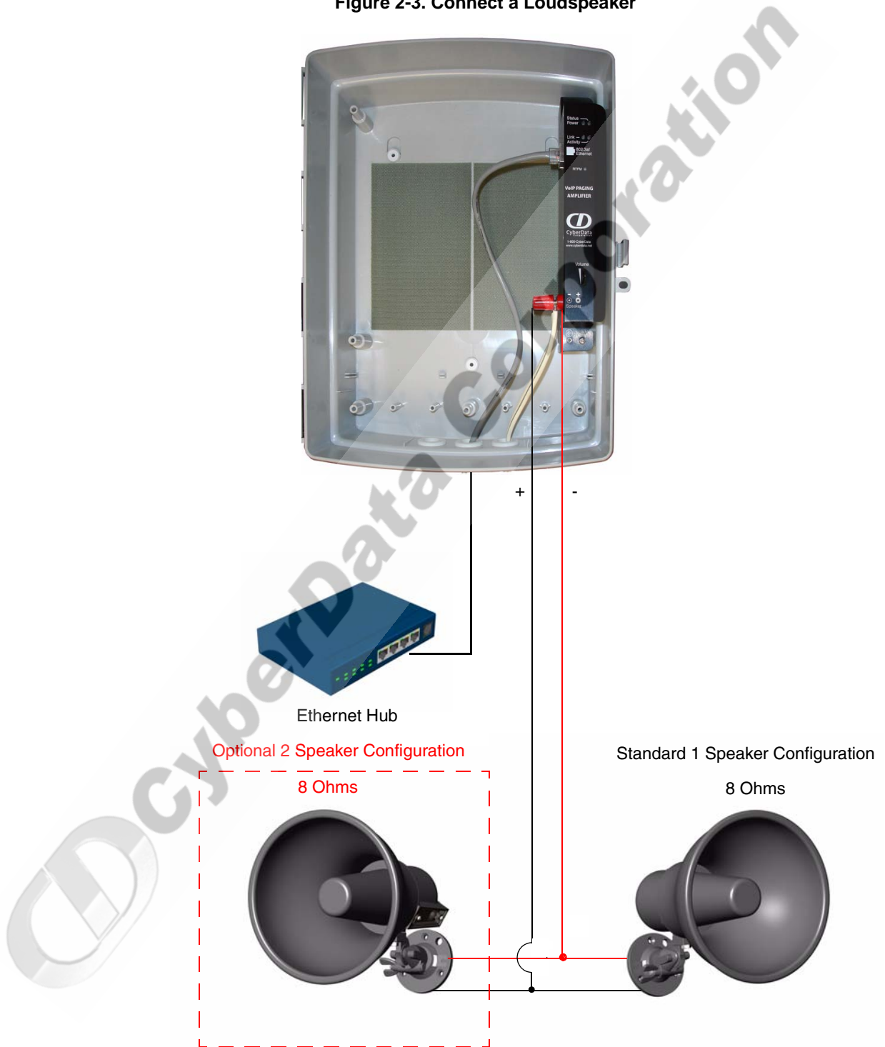
Figure 2-3. Connect a Loudspeaker
